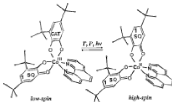
図14 コバルト錯体 [\text{Co}(\text{phen})(3,5\text{-DBSQ})_2] \text{C}_6\text{H}_5\text{CH}_3 の valence tautomerism.
